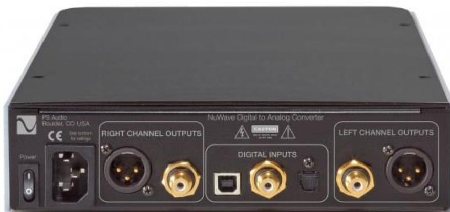
Besides USB, the NuWave also offers alternative digital connections (TOSLINK optical, or RCA coaxial) but for connection to a computer it is the USB port that is recommended. It features an XMOS based,
